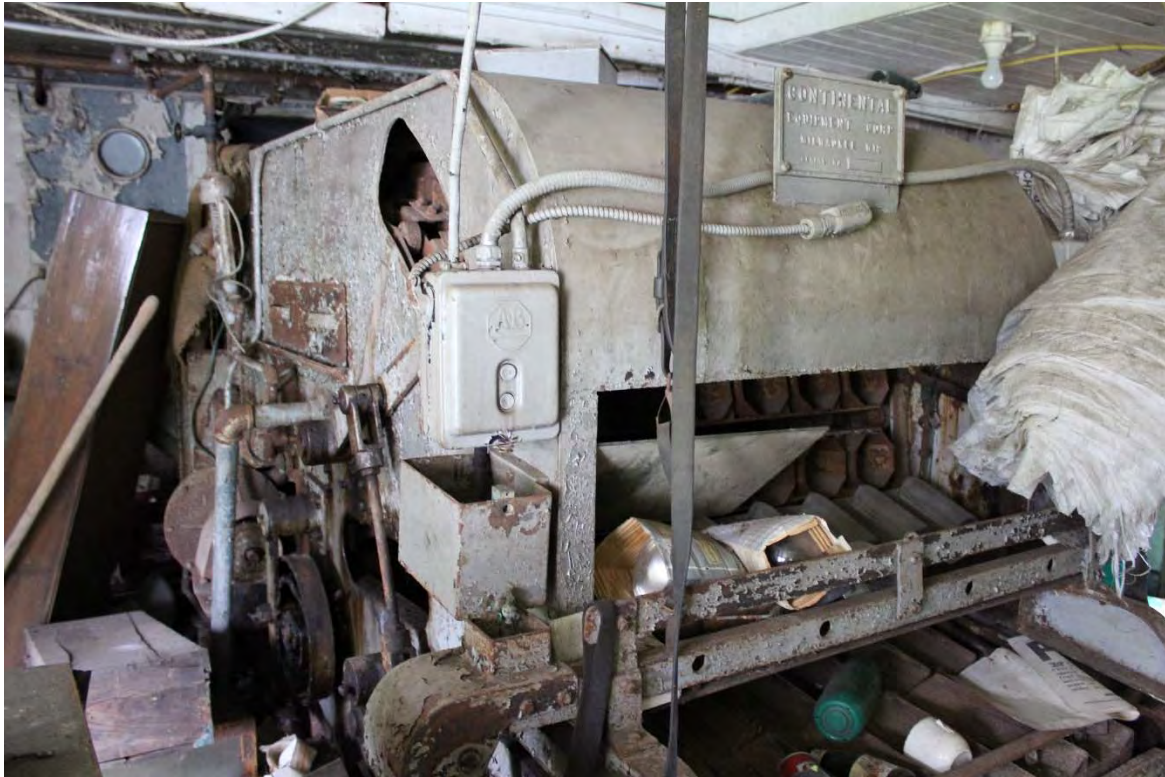
Photo 35. View of mechanized bottling machine.
